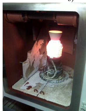
Fig. 4. a) insulated ceramic mold, b) mold after pouring
