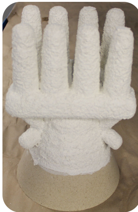
Fig. 1 Shell mold fabricated through the “dip and stucco” technique
