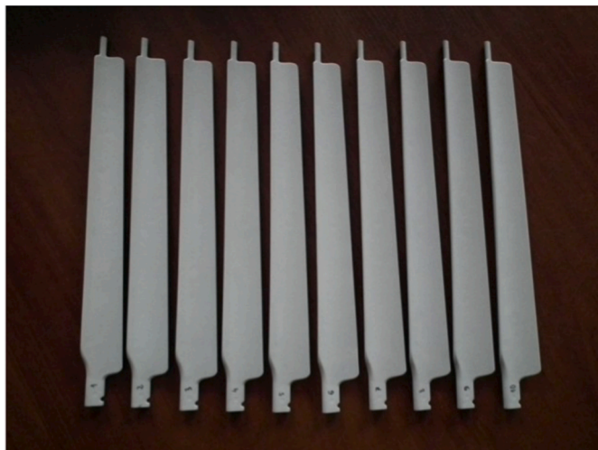
Fig. 3. The cores debinded for 8 h after the final sintering.
