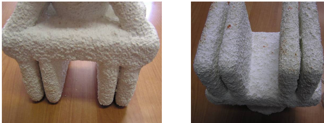
Fig. 3. Ceramic mold a) with 9 ceramic coatings, b) with 11 ceramic coatings
