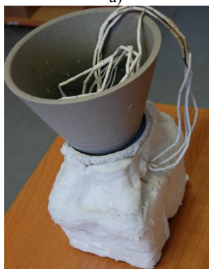
Fig. 4. a) insulated ceramic mold, b) mold after pouring
