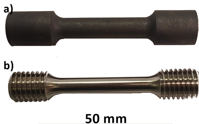
Fig. 2. Geometry of prepared element after: a) excision b) machining
