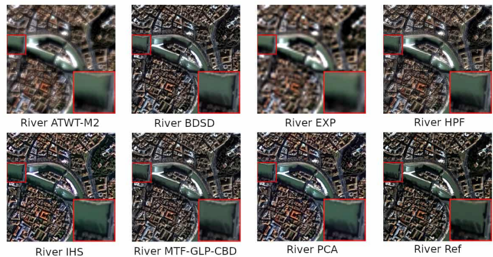
Figure 8. TC images obtained with PS methods compared with the reference (Ref) for IKONOS Rome River scene.
