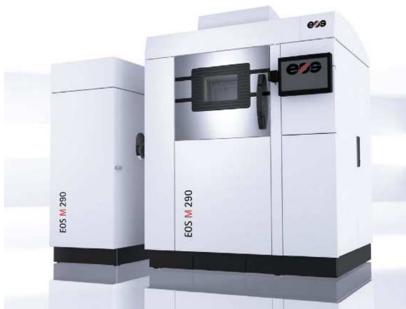
Rys. 4.32. System M290 DMLS oparty na PBF firmy EOS
