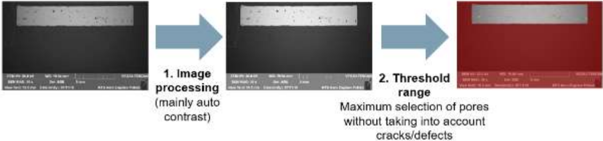
Figure 17 IMS analysis of microporosity in the SiC/SiC composite
