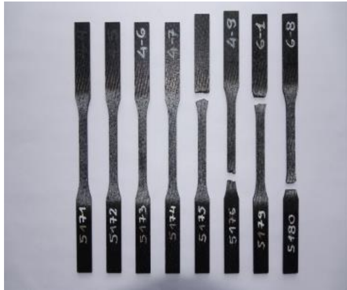
Figure 64 Samples after creep testing in the temperature 980 °C
