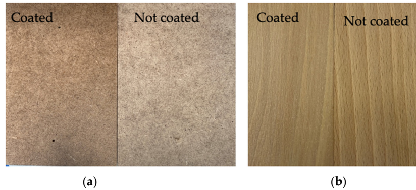
Figure 5. MDF (a) and woodplates (b) coated using L-IGKFX/HEA.
